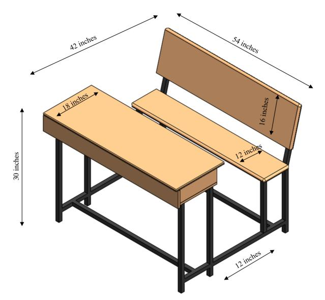
Size of the Legs: 1.25"X1.25" Material of the Legs: Mild Steel All plates: 19 mm Plywood with 0.8 mm Sunmica
