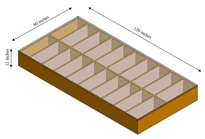
**Structure plates:** 19 mm Plywood **Top Plate:** 19 mm Plywood with 0.8 mm Sunmica
